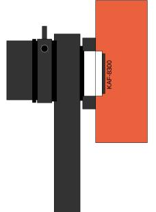
Distance from chip to M48 winding of OAG ~ 41mm
